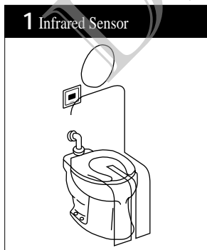
The infrared sensor detects a user sitting on the toilet seat.
