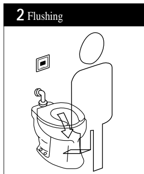
After using over 5 seconds, when a user leaves the fixture, the sensor automatically sends a signal to the operating unit to activate the flush valve.
